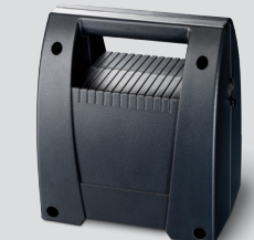
Battery pack Rated voltage: 12 V DC, rated capacity: 15 Ah, service life: 40 days for a maximum of 4 openings a day and a temperature of 20° C, temperature range: - 15 ° to + 45 °C, integrated charge controller for mains power pack • Suitable for: Novomatic 423 Accu
